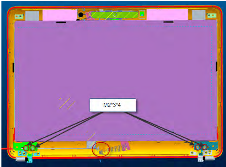
Figure 4-14-2 Remove screws securing the LCD
