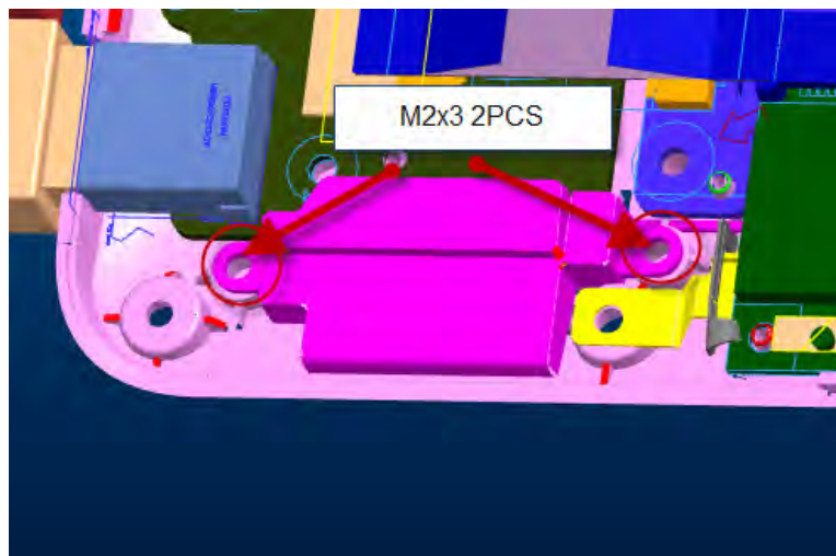
Figure 4-17-1 Remove the securing screws at left side.
