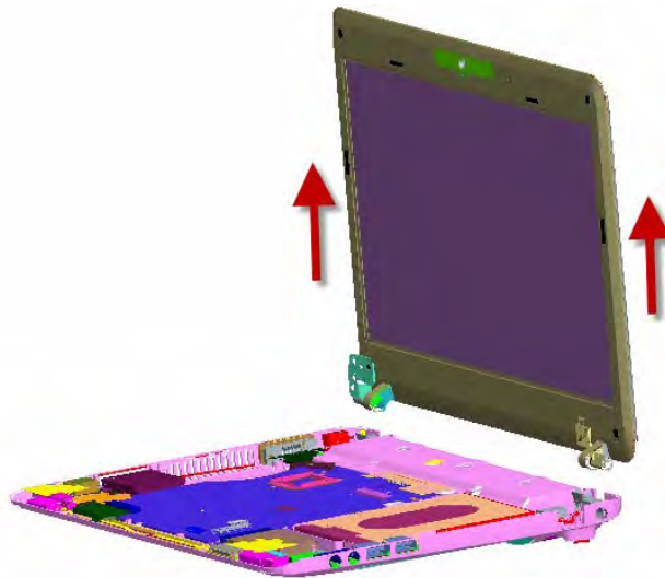
Figure 4-8-9 Remove the display assembly
