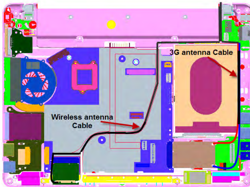
Figure 4-8-12 Arrange and connect Wireless LAN cable and 3G
