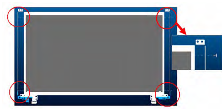
Figure 4-14-5 Remove the LCD hinge
