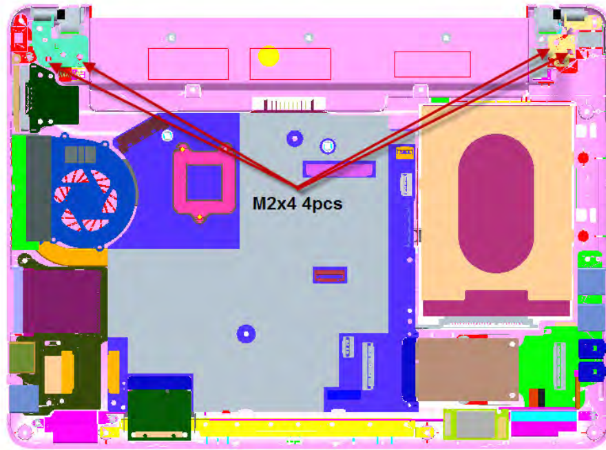
Figure 4-8-8 Remove the hinge screws
