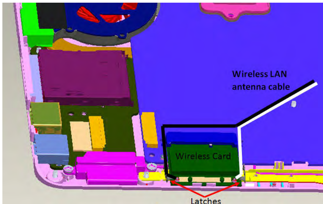
Figure 4-6-1 Remove a wireless LAN card
